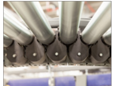
Rollers with clasps for fast replacement
