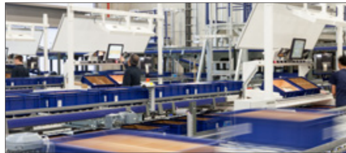
Maximum performance: Streamline achieves a throughput of up to 3,500 containers per hour
