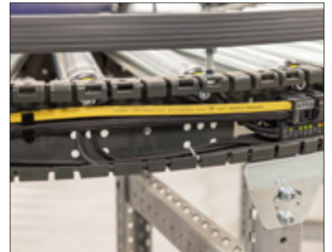
Smart control concept: the proven AS-i bus system
