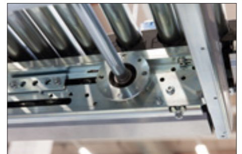
Self-tightening tension unit at roller conveyor system
